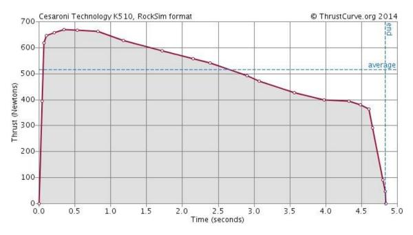
This is an accurate measure of the thrust over time graph for the K-510 Classis motor made by Cesaroni Technology Incorporated.
