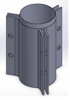
The entire payload will be the dimensions of a coupler tube, so the entire piece will slide easily out of the back half at apogee. Both ends will have a U-Bolt attached directly to the bulkheads, which will attach the payload to the drogue parachute and the rest of the rocket components. The payload will eject at apogee during the first stage of ejection, at which point the drogue parachute will also deploy.
