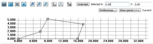
Our fins will be made of ultem, and 3D printed by TE Connectivity. They will be placed at the bottom of our rocket, and they will be 120 degrees apart from each other. They will be screwed onto the body tube. The screw will go through the body tube, and into wood that is on the inside of the body tube. This will keep it secure to the body tube, and prevent it from coming off.
