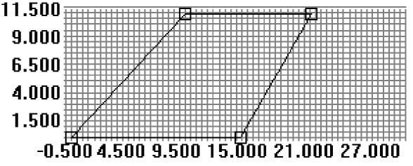
CG is 79.94 inches from the front end and CP is 101.14 inches. This is 21.2 inches apart, and based on the diameter of the rocket, this gives a margin of 1.86.
