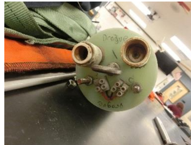
Ejection Wells for Drogue
