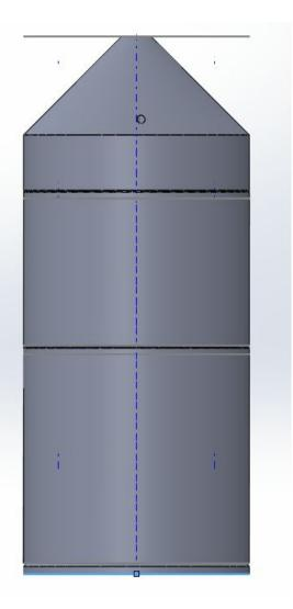
This shot shows a side view of the nosecone and payload air chamber. You can
